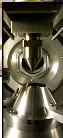
Above: A view of the JENSA system as installed in the ReA3 hall. Visible on the right is the dedicated beamline, with the target chamber, series of vacuum pumps, and the control panel. On the left is the industrial compressor, used to return the gas to the high pressures required to feed the jet. Left: A close-up photograph of the JENSA jet nozzle and gas receivers inside of the target chamber. Detector mounts are visible in the background.
